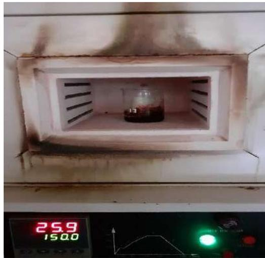
Gambar 5.14 Proses Kalsinasi  $\text{BaFe}_{12}\text{O}_{19}$
