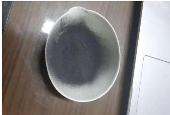
Gambar 5.18 Hasil *Sintering* Material temperatur 1000°C
