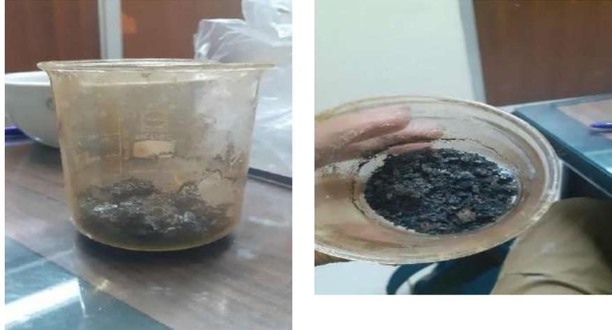
Gambar 5.15 Hasil Kalsinasi  $\text{BaFe}_{12}\text{O}_{19}$
