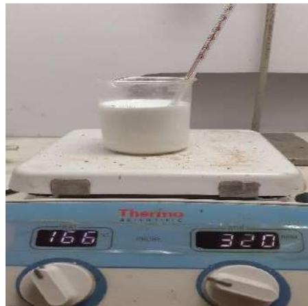
**Gambar 5.2** Sintesis Material  $\text{BaTiO}_3$
