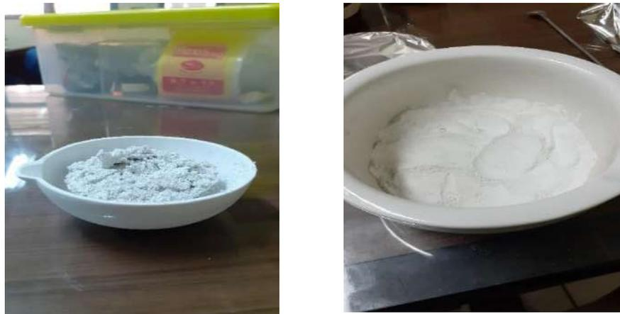
Gambar 5.4 Hasil *Sintering* material  $450^\circ\text{C}$   $\text{BaTiO}_3$
