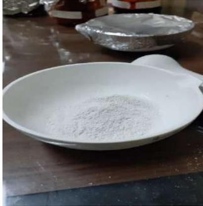
Gambar 5.5 Hasil *Sintering* material 700°C BaTiO<sub>3</sub>
