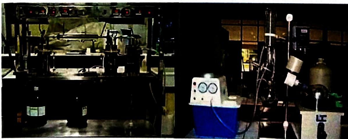
Fig 4. The bubble column reactor setup and rotary evaporator for final product separation from methanol
