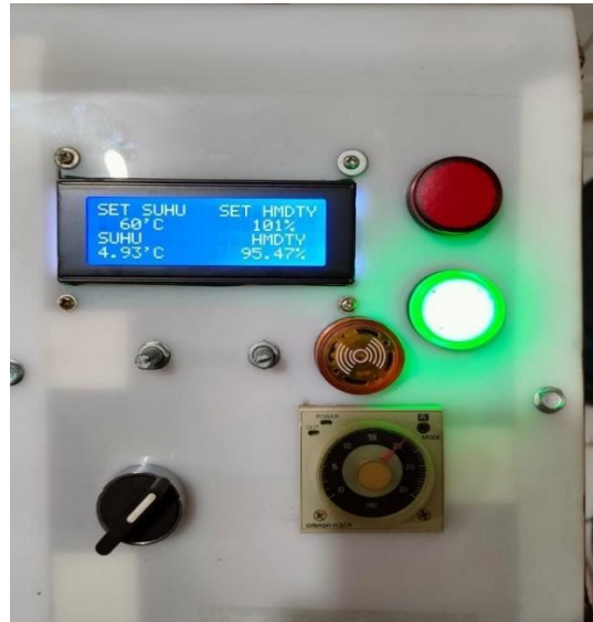
Gambar 4. 41 Tampilan instrumen panel kondisi selector switch ON
