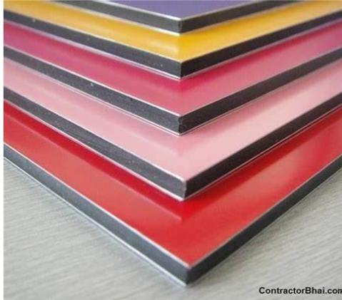
Gambar 7.5 Material Aluminium Composite Panel
