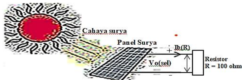
Gambar 3.8. Tegangan V_{O(sel)} mensuplai beban listrik resistor R = 100 \Omega
