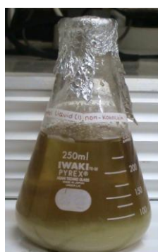
Fig 9. Reactant in the bubble column reactor after 3 hr reaction at 250 °C reaction condition
