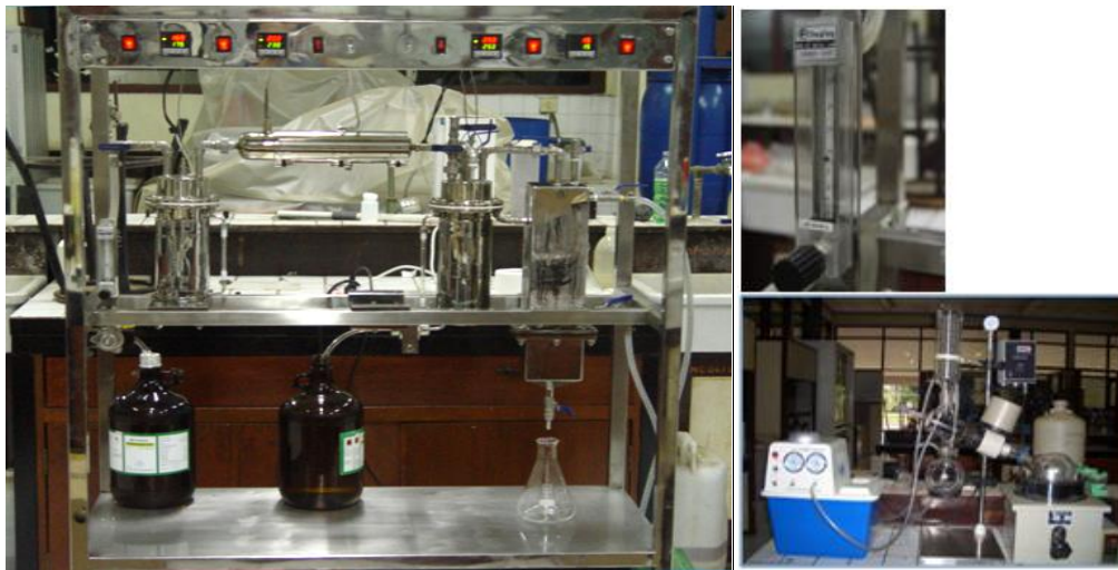
Fig 3. The bubble column reactor setup and rotary evaporator for final product separation from methanol
