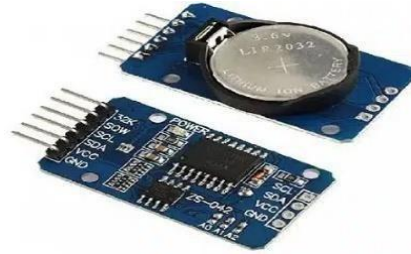
Gambar 2. 22 RTC DS3231 (Sumber: https://www.watelectronics.com )
