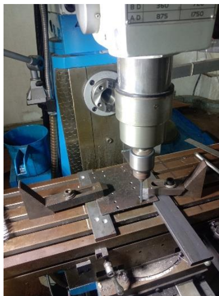
Gambar 13. Proses pengeboran ( drilling )
