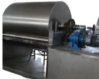
Gambar 4. 12 Rotary Dryer (RD-01)
