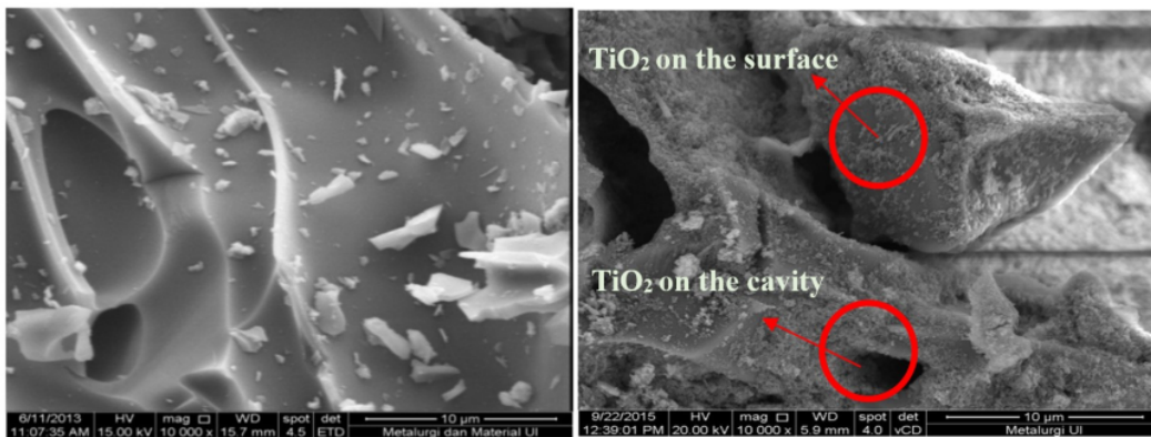
Figure 2. FE-SEM images with magnification of 10000X for (a) Pumice stone/PS; (b) PS-TiO 2 .
