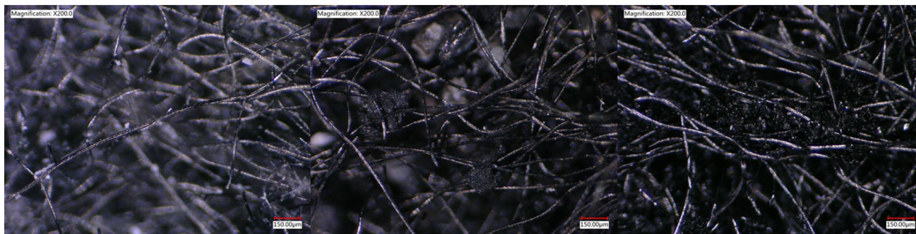
Fig. 3 DOM for CF (left), CF/CP (middle), and CF/AC (right) at 200× magnification
